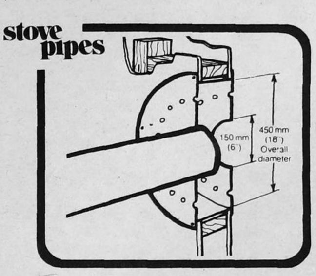
**Stove Pipes** — Make sure that your stove pipes are in good condition and cleaned regularly. Here again creosote buildup can present a fire hazard. To minimize buildup, pipes should be as short as possible.
