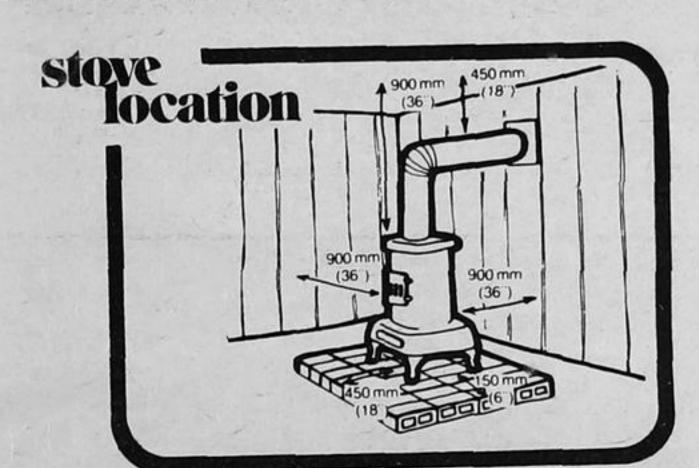
Stove Location — The stove (or metal fireplace) must be kept well clear of walls and partitions. If the wall or partition is not protected, the stove should be at least 36 inches away. If a metal and asbestos shield is used, with at least one inch clearance between the shield and wall, the stove can be located as close as 18 inches. Anything less is unsafe. Similarly, combustible furniture and other flammables should be kept at least 36 inches away from a stove or fireplace.
