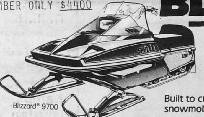
Wind tunnel-tested aerodynamics; carbide runners for high-speed cornering; a massive 534 racing-type, liquid-cooled Rotax\* engine; the "super torque" of an asymetrically-timed rotary valve...
