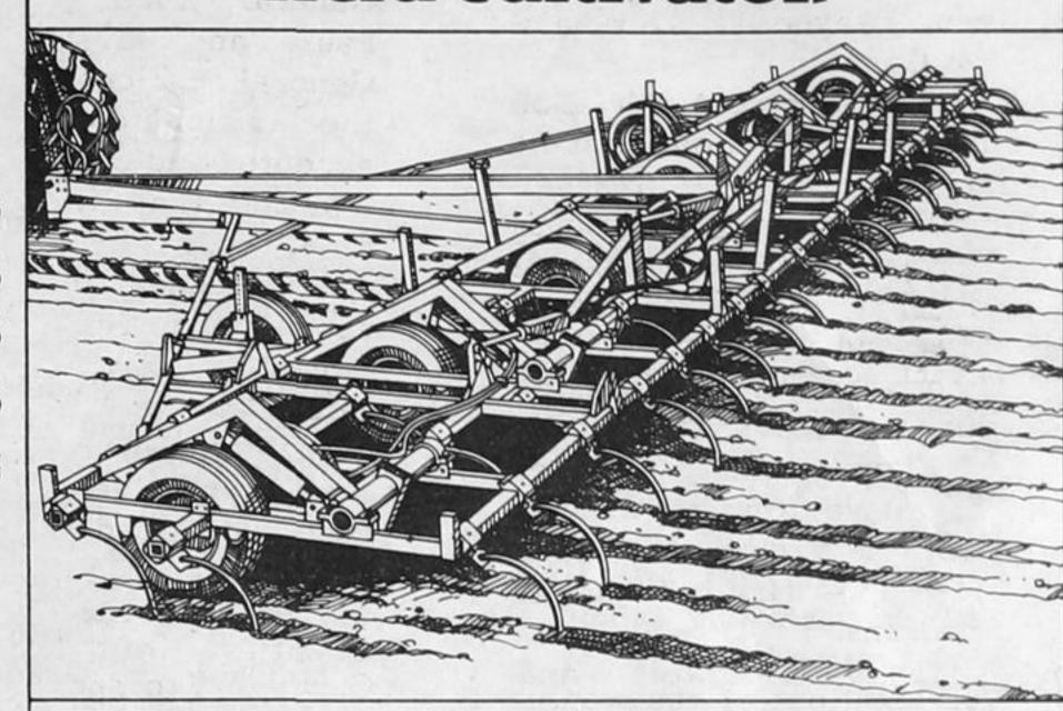
From 10½ to 61 feet, you'll have the best engineering working for you. Exclusive rubber elastomer clamps promote vibrating action in shanks to help shatter soil and leave a level surface. Does more work with one pass over the field.
