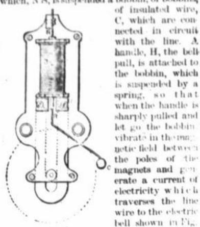
C, which are connected in circuit with the line. A. handle, H, the bellpull, is attached to the bobbin, which is suspended by a spring, so that when the handle is sharply pulled and let go the bobbin vibrate in the manetic field between the poles of the magnets and gove erate a current of electricity which traverses the line wire to the electric
