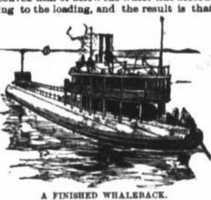
when they strike the upright sides of a common vessel. The bow end is sharp and circular and the stern rounded in a similar way. With all these advantages Captain McDougall thinks that seasickness can almost entirely be avoided, but at present his designs have reference only to the cheapening of freight transportation. In towing barges the saving is enor
