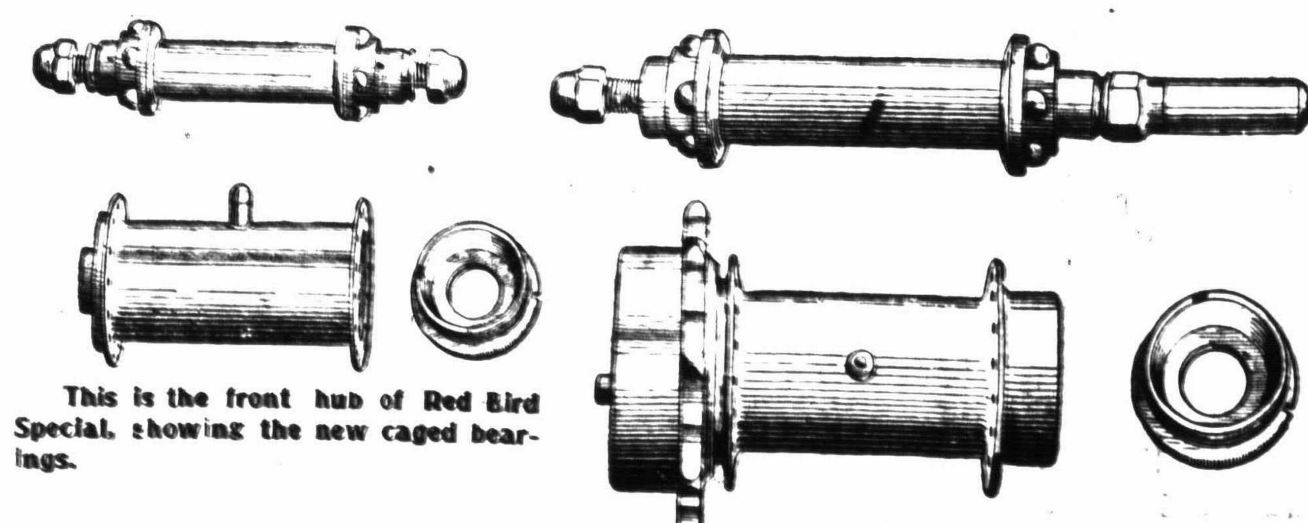
Rear Hub of Red Bird Special showing William automatic brake and new caged bearings.
