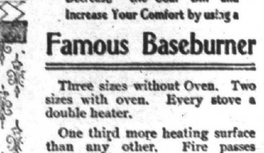
through three flues, while other stoves have only two, and thus securing one third more heat from the same fuel. Parlor stoves draw the cold air off the floor. Removable firepot; flat or duplex grates; removable nickel jackets. The oven bakes perfectly.
