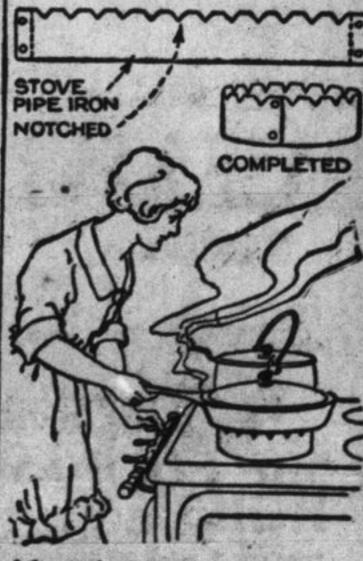
of the notches will light the gas when the tap is opened. The use of such a ring concentrates the heat under the ve
