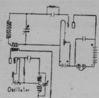
connected across the grid and plate coils of the oscillator. Oscillations will of course be induced in the secondary circuit by the oscillator and will be of maximum strength when the secondary is in resonance, other things being equal. The coupling between the oscillator and the secondary circuit will also of course affect the strength of
