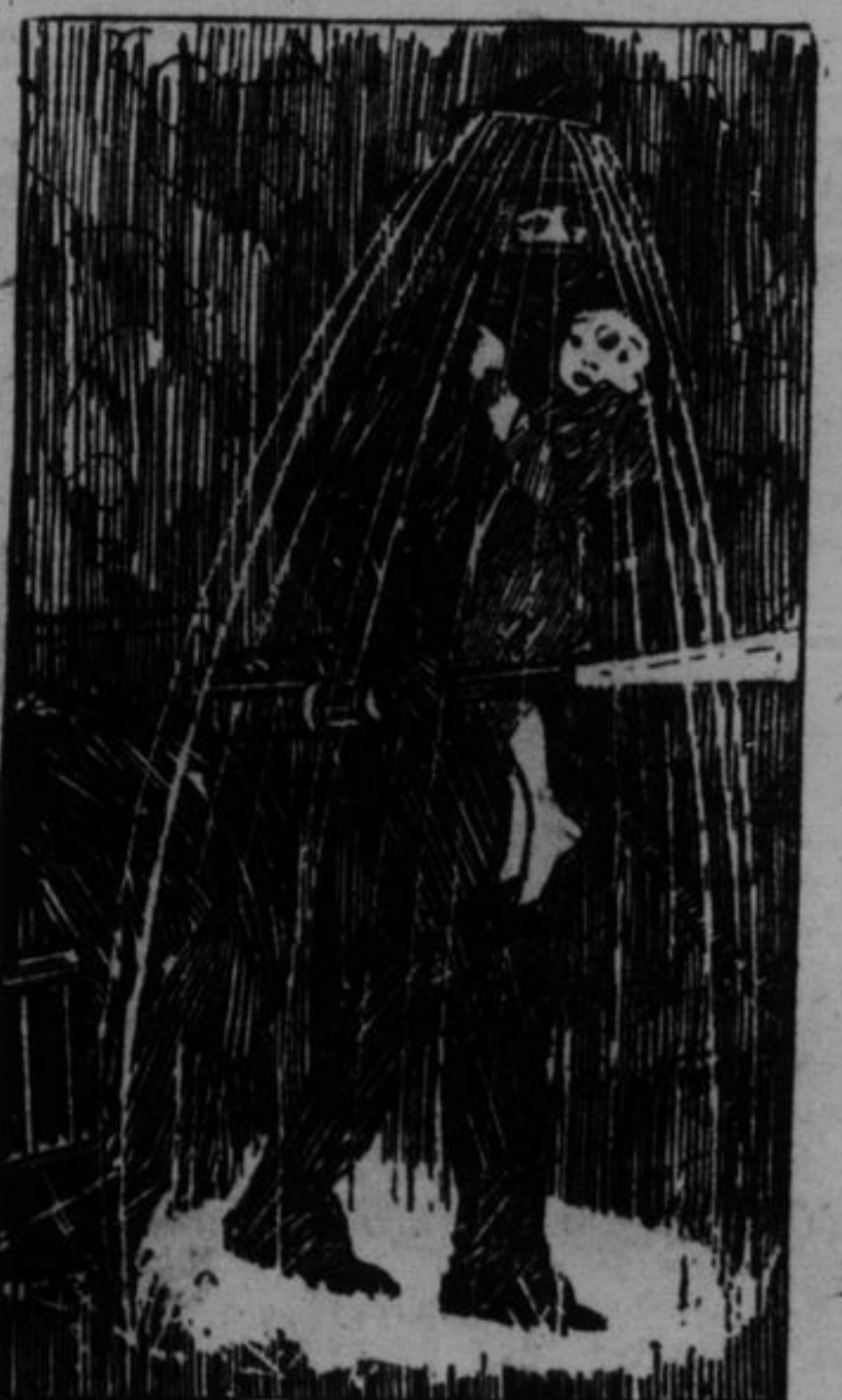
The Latest Fireman's Suit Sprays a Sheet of Water Down Between the Inner and Outer Coverings, as Well as Providing an Outer Water Curtain Which is Supplied from the Main Fire Hose.
