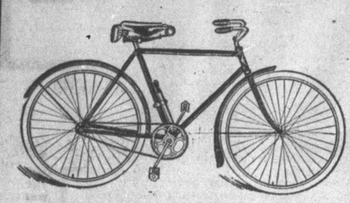
Here's a fully equipped Indian Bicycle with Dunlop style tires, coaster brake, roller chain, comfort pedals, motorcycle saddle and extension handle bars.
