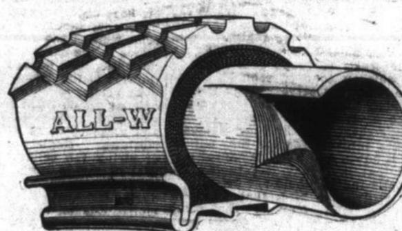
This is a section of both Tube and Tire. The Inner Tube is pictured to show the layers which compose it. In completed Tubes these layers, of course, are vulcanized together into one solid rubber Tube.
