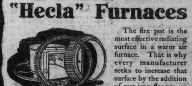
The fire pot is the most effective radiating surface in a warm air furnace. That is why every manufacturer seeks to increase that surface by the addition of cast iron flanges, or
