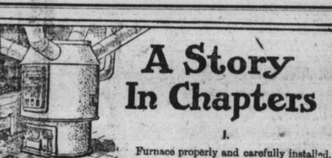
With great case water is placed in waterpan, drafts opened and coal fire started. Fire soon burns up brightly, drafts are closed and checkdraft opened. Immediately heat-power begins to penetrate dome and radiator surrounding dome. The incoming cold air immediately receives the energy of this heat-power, and by natural law ascends up the hot-air pipes, thence to rooms. No gas escapes into cellar or rooms because there is an automatic gas damper providing for its escape
