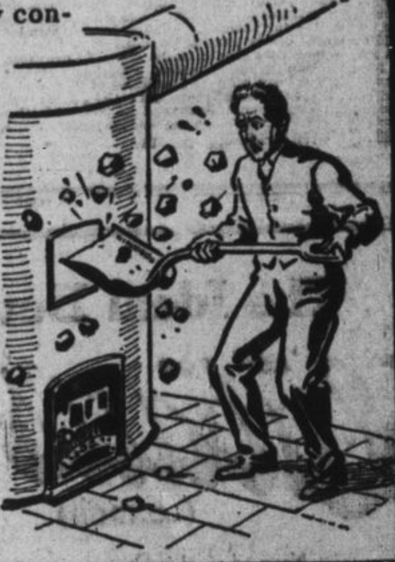
The Common Way of Distributing Coal on the Floor.
