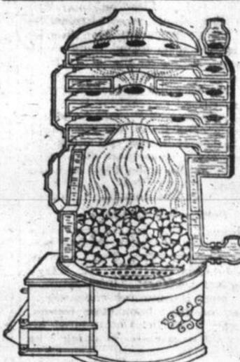
THE Oxford Hot Water Boiler takes advantage of every known scientific point which will increase the generation and distribution of heat. We have increased its power enormously by making the walls of the fire pot slant inwards above the fire. This gives a greater surface for the direct action of the rays of heat.
