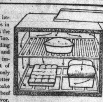
ents produced the oven-heating system of the Oxford Range
