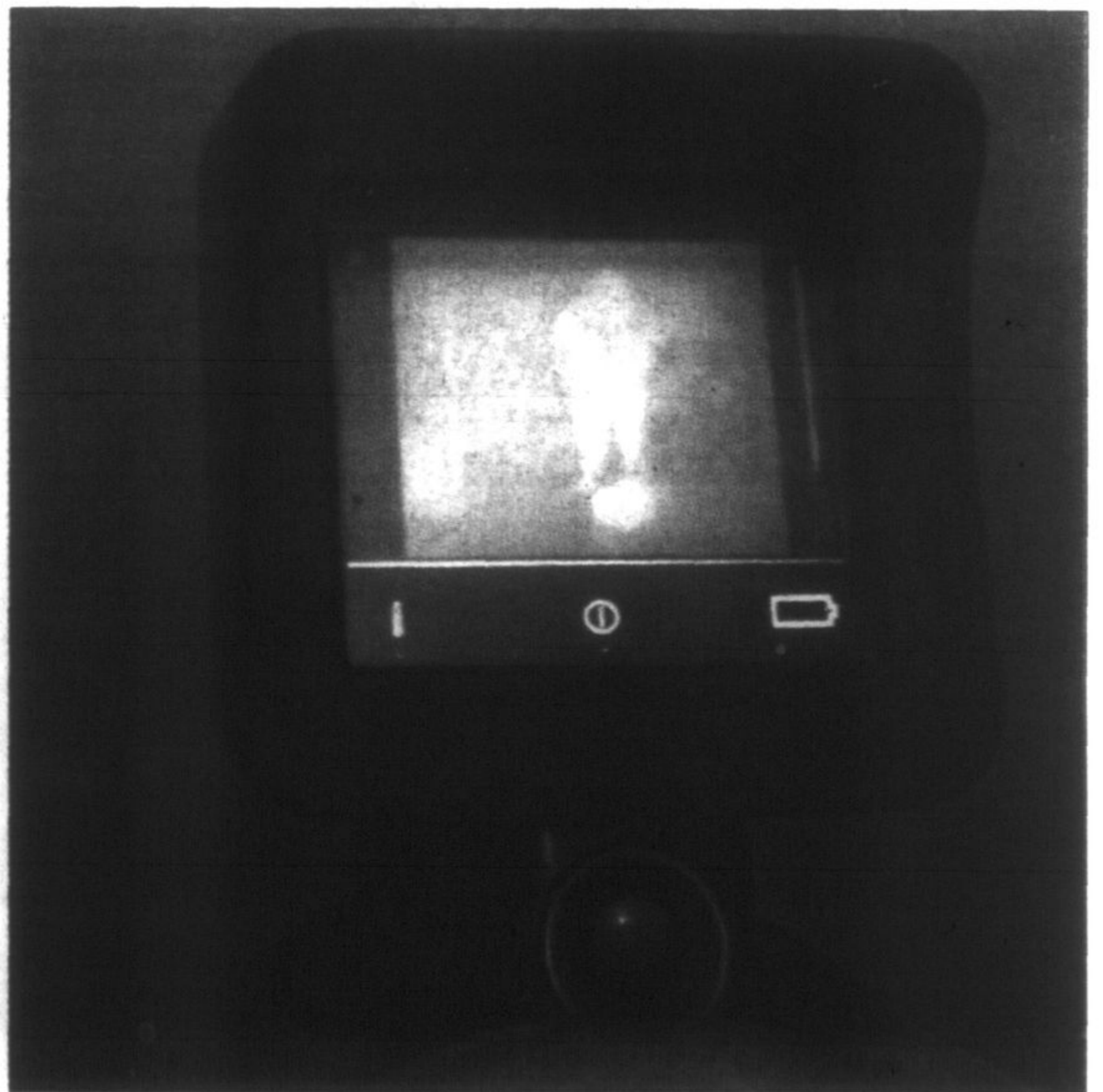
A thermal imaging camera detects items based on temperature. "It's a great tool that assists firefighters during search and rescue as well as fire extension in hidden areas such as walls and ceilings," said Fire Prevention Officer Jeff Bignell. The new recruits graduated from training at a ceremony Feb. 20.
