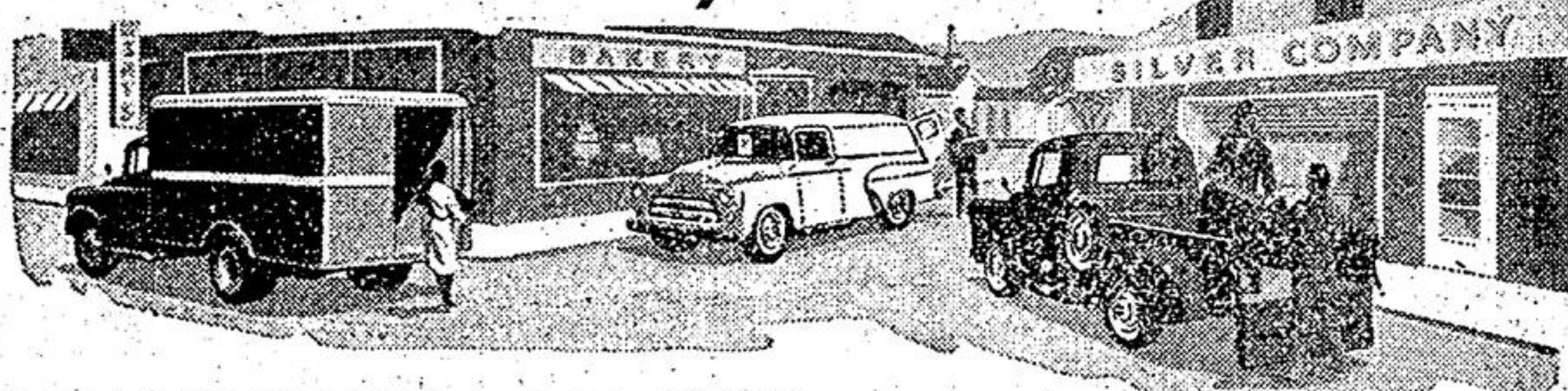
"A" model Chassis and Cab with Van Body—15,000 lbs. G.V.W. "B" model Panel—5,000 lbs. G.V.W. "C" model Express—6½-foot body, 108" wheelbase—5,000 lbs. G.V.W.
