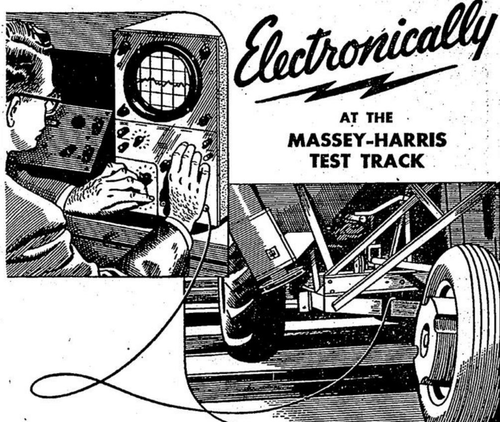
As Massey-Harris machines go "over the bumps" on the test track, the inside story of strains and stresses set up in frame members and working parts is recorded by special electronic apparatus.
