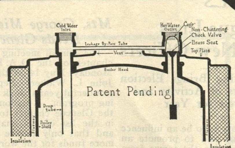
This Is the EverHot Leakage By-Pass. No Other Heater Has It. It Saves Gas
