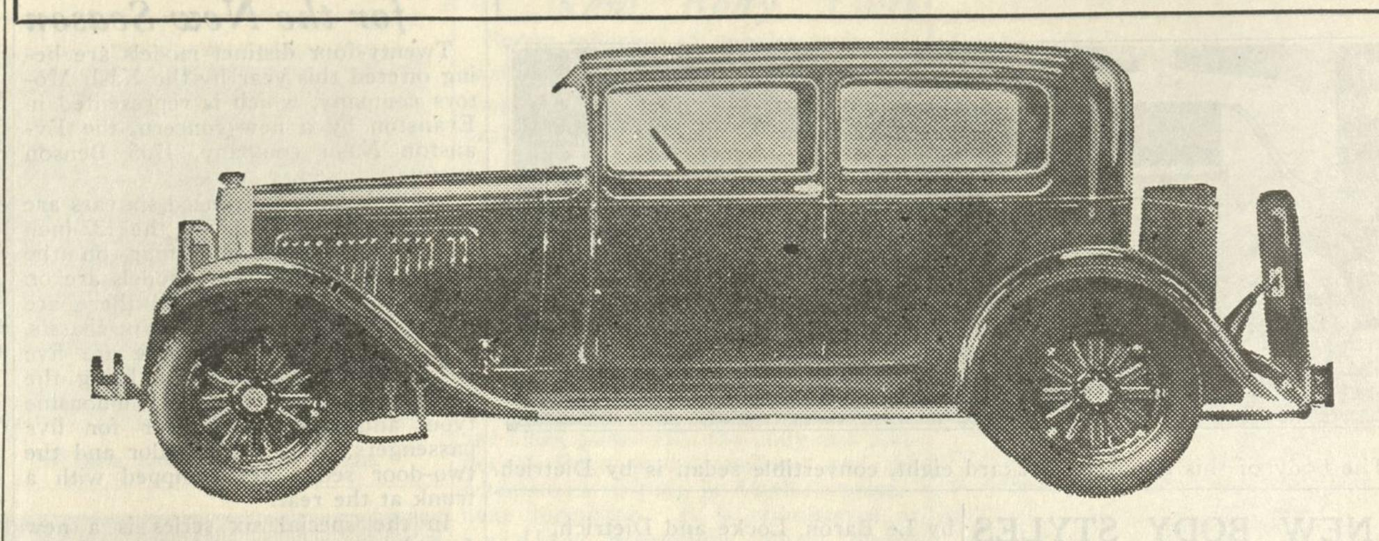
This is the Victory Six brougham. It is one of the new Dodge Brothers sixes which are making automobile history because of their unit construction of body and chassis and because of their double wall of steel in body construction.
