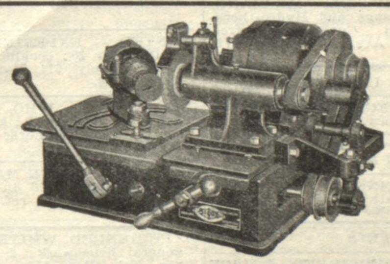
Let me reface, reseat, and grind your valves with the new Sioux Valve Machine. By virtue of this machine we can give the best results possible to obtain, with no extra charge.
