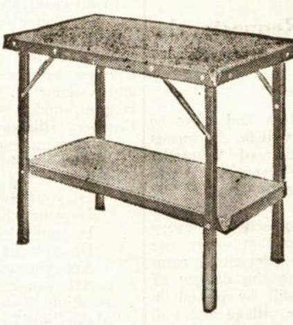
CONSTRUCTION-Top and shelf of heavy fibre board and the supporting side rails of SEASONED HARD WOOD, depth 11/2", width 7/8". The top also has one wood center brace, and the shelf three wood braces running crosswise to carry the extra weight of the batteries.
