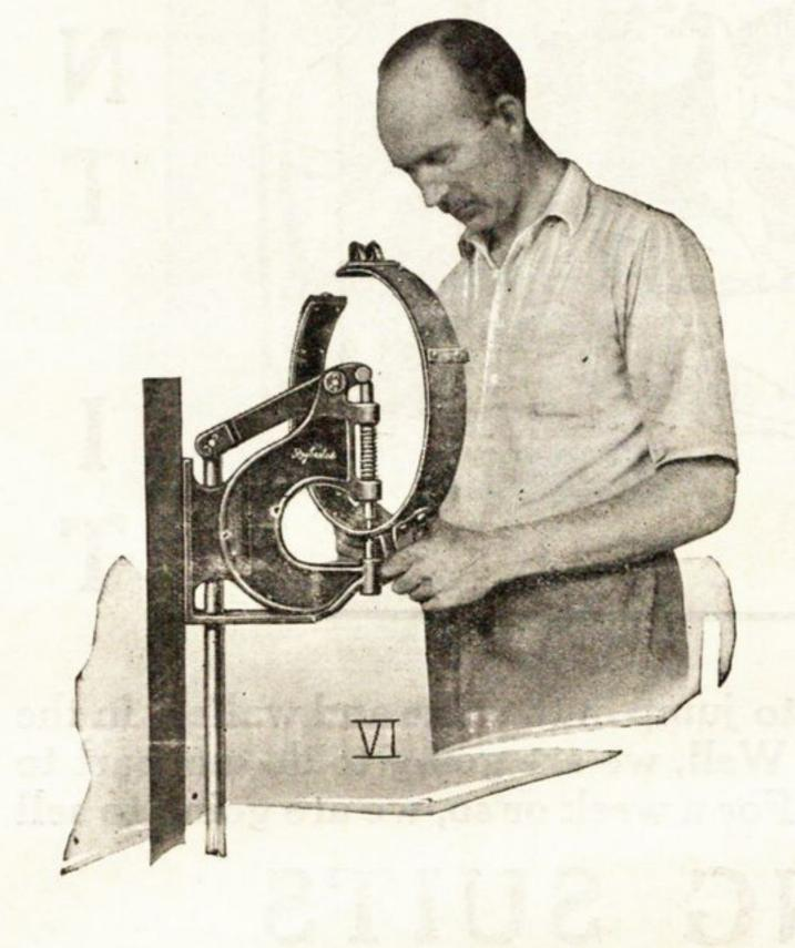
This is one of our brake relining machines. It punches out the old rivets and rerivets the new ones. It saves time and produces a "factory" job. Have your brakes relined by a service station which is properly equipped.
