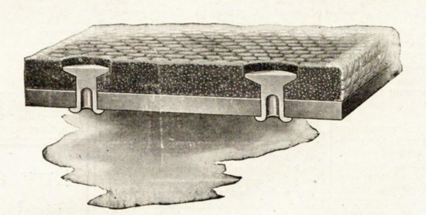
Correct method for attaching Brake Lining with Tubular Brass Rivets Properly Countersunk.
