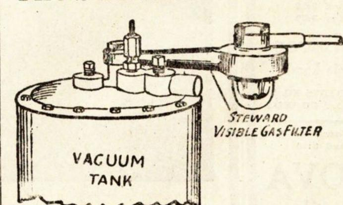
1 OU can instantly see how the I gasoline comes in through the intake tube, flows down into the glass trap cup, and then goes upward through the mesh and out through the shank to the vacuum tank.
