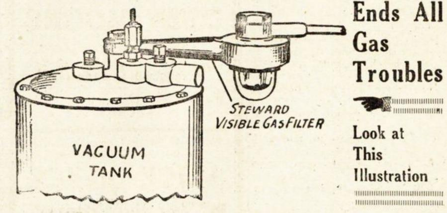
You can instantly see how the gasoline comes in through the intake tube, flows down into the glass trap cup, and then goes upward through the mesh and out through the shank to the vacuum tank.
