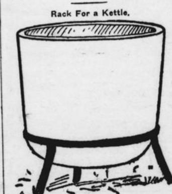
and one-half inch thick and long enough to make a hoop to fit your kettle, make a hoop out of it and weld it together, then take three pieces of iron about an inch in diameter and about a foot long and weld to the hoop for legs, The legs can, of course, be made any shown are about a foot long. This gives plenty of room for wood, and there is no danger of the kettle falling. Another plan may be to use gas pipes with the legs set in the pipe.-Iowa Home-
