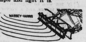
It has great capacity, nevertheless, and is strong and well-made. It drops back from under the sheaves | self. when dumping, without damaging the heads of grain.
