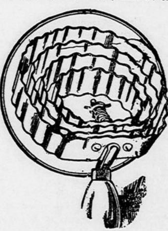
side by a metal binder, which also acts as a handle. The greatest advantage claimed for this idea is that there are no lodging places for the germ laden dust which it extracts from the animal's hair, and any such accumulation must pass right through it, and for the particular horse owner it offers opportunities for further precautions against contamination by washing in water. This device sousca around in some soapy water would be thoroughly cleansed.
