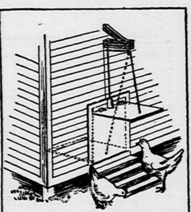
strength to give way under the weight of a hen. A door is next made and hinged at the top as shown. To this door is fastened a rope leading to a weight that is heavy enough to lift the door. A small strip of wood is nailed across the front of the hinged platform, completing the work. The details are clearly shown in the sketch and require no further explanation.
