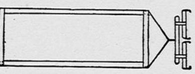
piece three feet long across each end. Fasten a hitch on one end and lay the harrow on it, teeth down. With this you can go through a gate almost too narrow for two horses. - Nebraska
