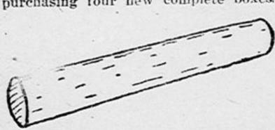
which would have cost me \$8, I bought a twenty foot piece of round shaft steel, seven-sixteenths of an inch in diameter, for 45 cents. This was cut into lengths corresponding to the old five-sixteenth inch rollers. These larger rollers took up all the wear, and I have practically a new disk for 45 cents and four hours' work.
