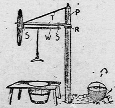
pole, over it and fasten securely with bolts or screws. This ring R and the iron pin are the means of supporting
