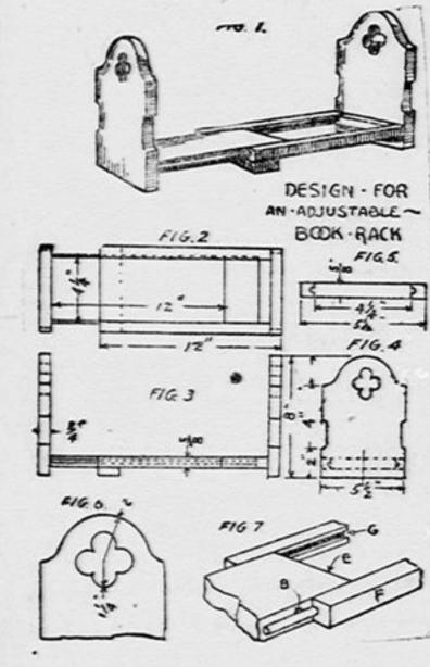
of the sides need not be fully drawn. Mark their centres only. Use a %inch bit in boring each of the four holes which form the completed hole.
