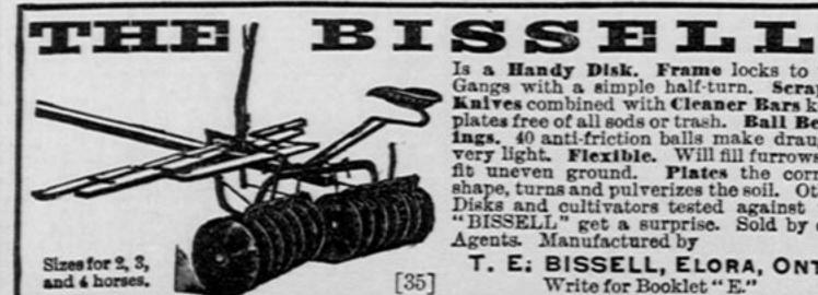
Is a Handy Disk. Frame locks to the Gangs with a simple half-turn. Scraper Knives combined with Cleaner Bars keep lates free of all sods or trash. Ball Bearings. 40 anti-friction balls make draught very light. Flexible. Will fill furrows or fit uneven ground. Plates the correct shape, turns and pulverizes the soil. Other Disks and cultivators tested against the "BISSELL" get a surprise. Sold by our Agents. Manufactured by
