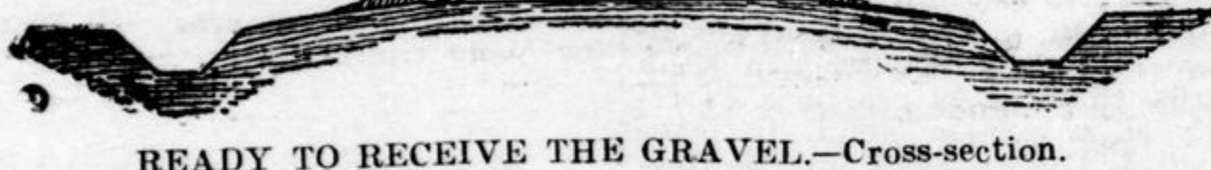
READY TO RECEIVE THE GRAVEL.—Cross-section. Showing earth shoulders as turned back by the grading machine.
