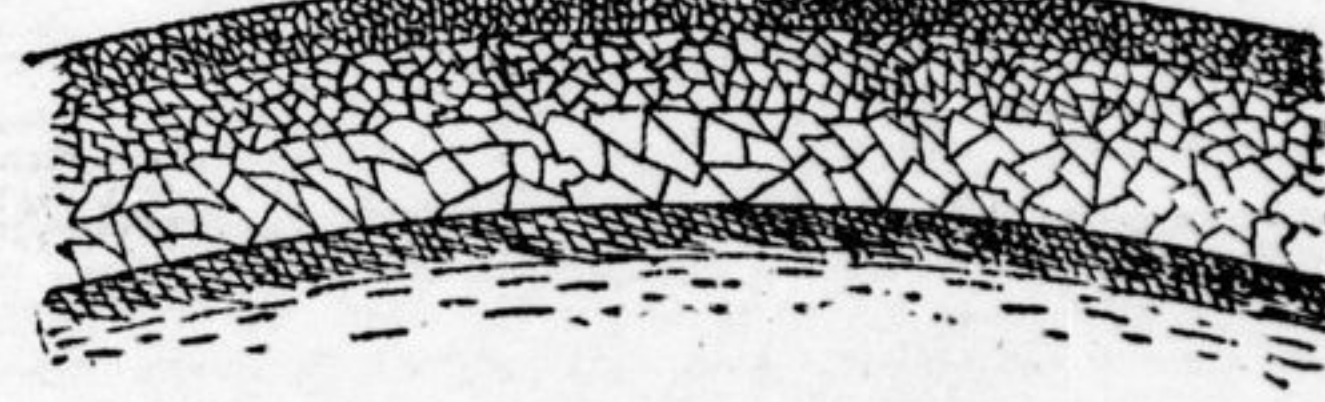
A GOOD ROAD COVERING.—Cross-section.
