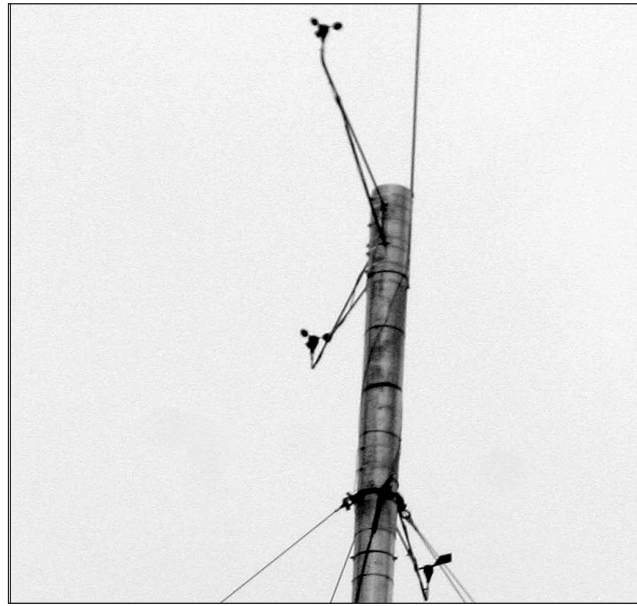
UNDER STUDY – Wind speed and direction are being measured by instruments atop 60-metre test towers, installed in numerous locations around Essex County by wind power development companies.
