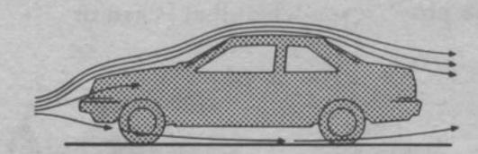
Tempo's clean-flowing lines are so effective, only six aero horsepower is needed to overcome wind resistance at 80 km/h. This very low drag factor means less fuel consumed. Not only that. Tempo's controlled air flow increases roadholding, improves handling, and reduces interior wind noise.
