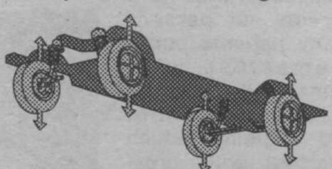
Tempo's front-wheel-drive design not only delivers extra tire-to-road traction, it gives you precise handling and tight, flat cornering. The new-design 4-wheel independent suspension allows each wheel to absorb road shocks independently. This smoothes out the ride and increases road-grip for extra safety.
