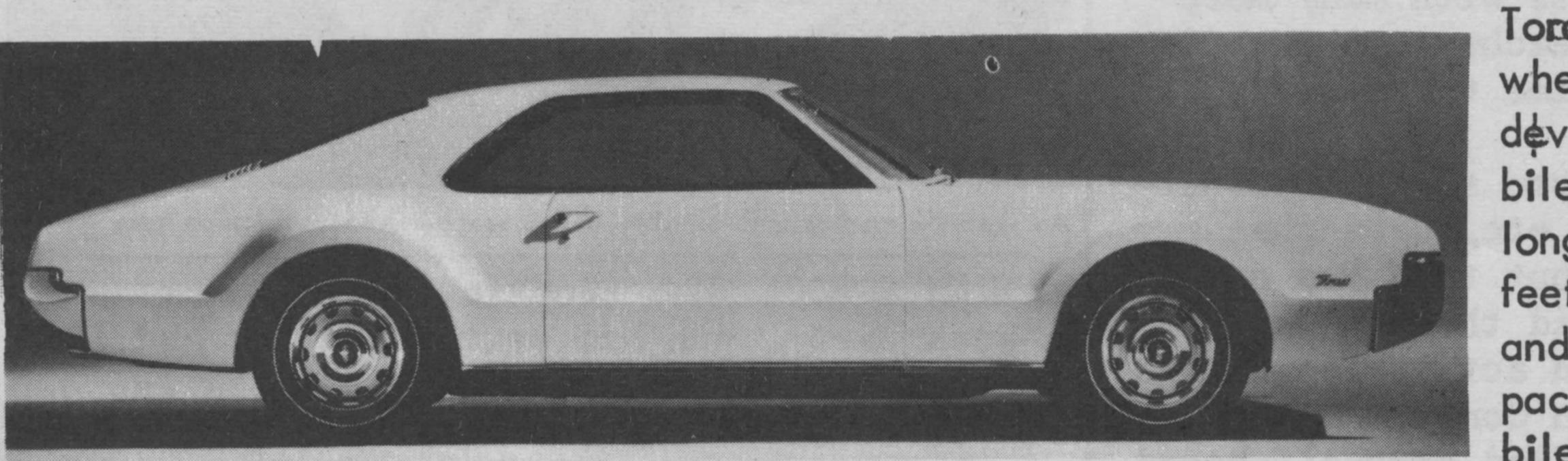
Toronado, Oldsmobile's frontwheel drive car, is the most radical development in production automobiles for 1966. It is 211 inches long, but only four and one-half feet high, and its fast - back design and long, low silhouette are the pace setters for the whole Oldsmobile line. Car height has been
