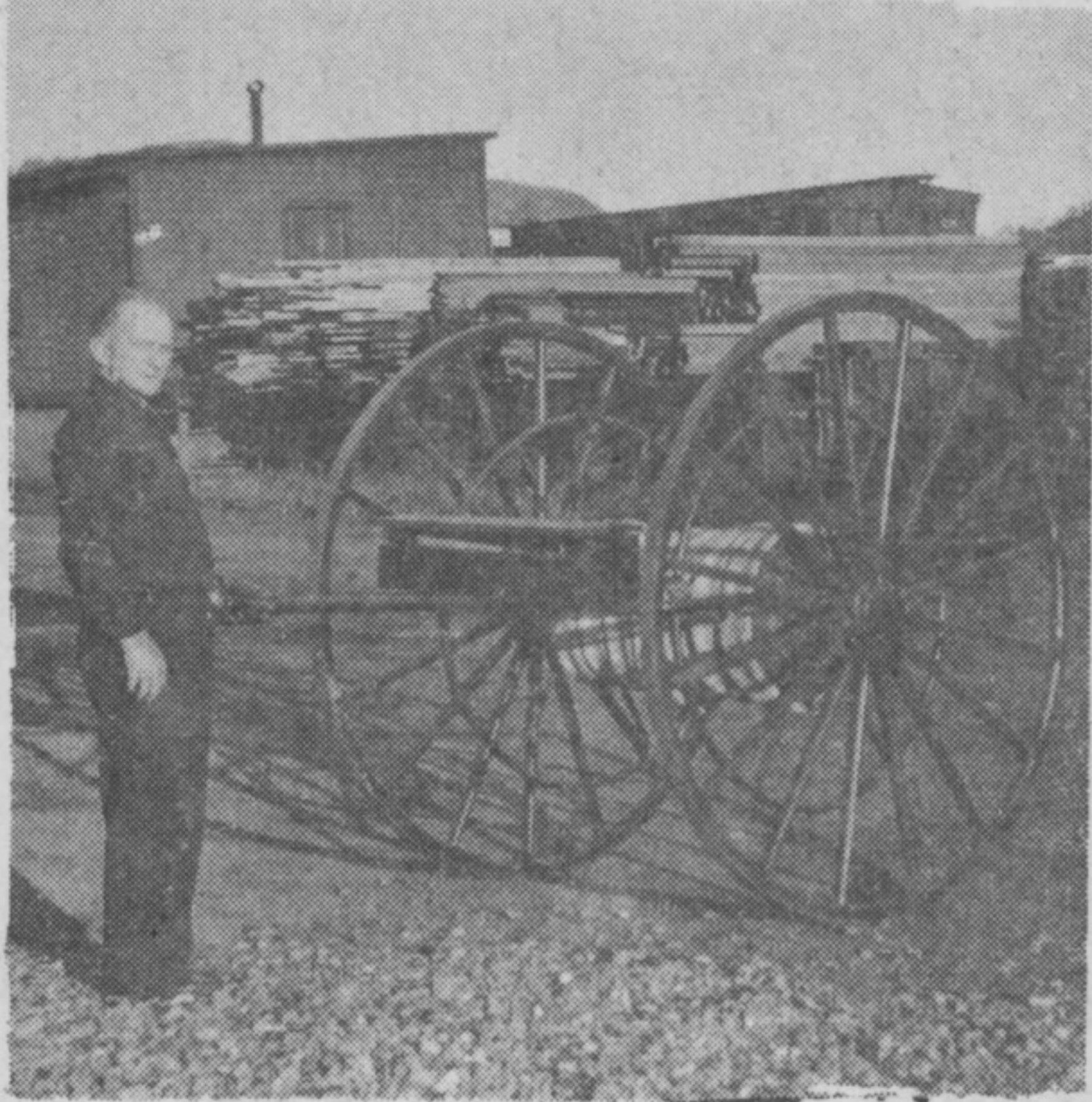
H. Stewart stands beside the first equipment - a hand drawn reel of hose, used on wheels in summer and on a toboggan in winter. Second picture - the remade car which was the first fire truck.
