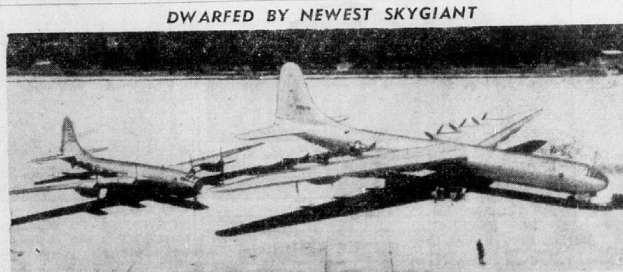
The sleek, silvered XB-36, U.S. newest and the world's largest land-based bomber, completely dwarfs a war-veteran B-29 Superfortress on the Convair, Fort Worth, Texas, division ramp. The giant plane completed its first test flight of 38 minutes as approving army air forces and air material command officers looked on. Wingspan of the XB-36 is 230 feet compared with 141 feet for the B-29; length of the new bomber is 183 feet, the B-29 99 feet; XB-36 has a maximum range with bomb load of 10,000 miles, the Superfort's is 4,100 miles with bomb load. The new plane's take-off power is 13,000 horsepower as compared to the B-29's 8,800.
