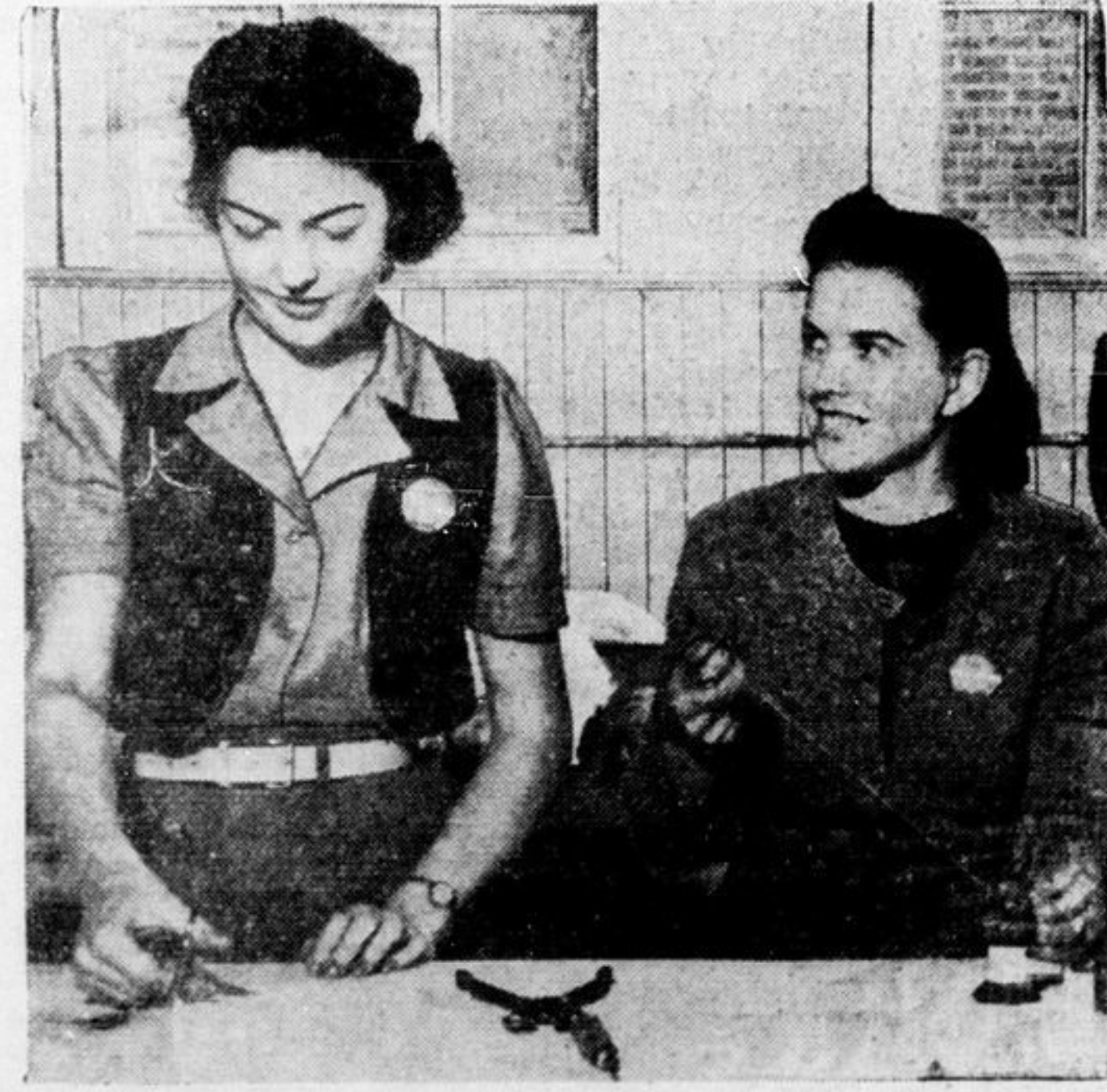
Canadian girls are shown above at work on the fabrics of the Norseman wings. These girls are doing their share in providing wings for the training of empire fledglings. The girls are cutting and sewing kapog used as insulation against cold, heat and sound in Norsemen "flying classrooms."
