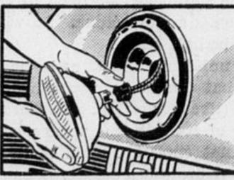
New Sealed Beam Safety Headlamps! They provide 50 per cent more illumination. The lens is sealed to the reflector, keeping dust and water from reflector.
