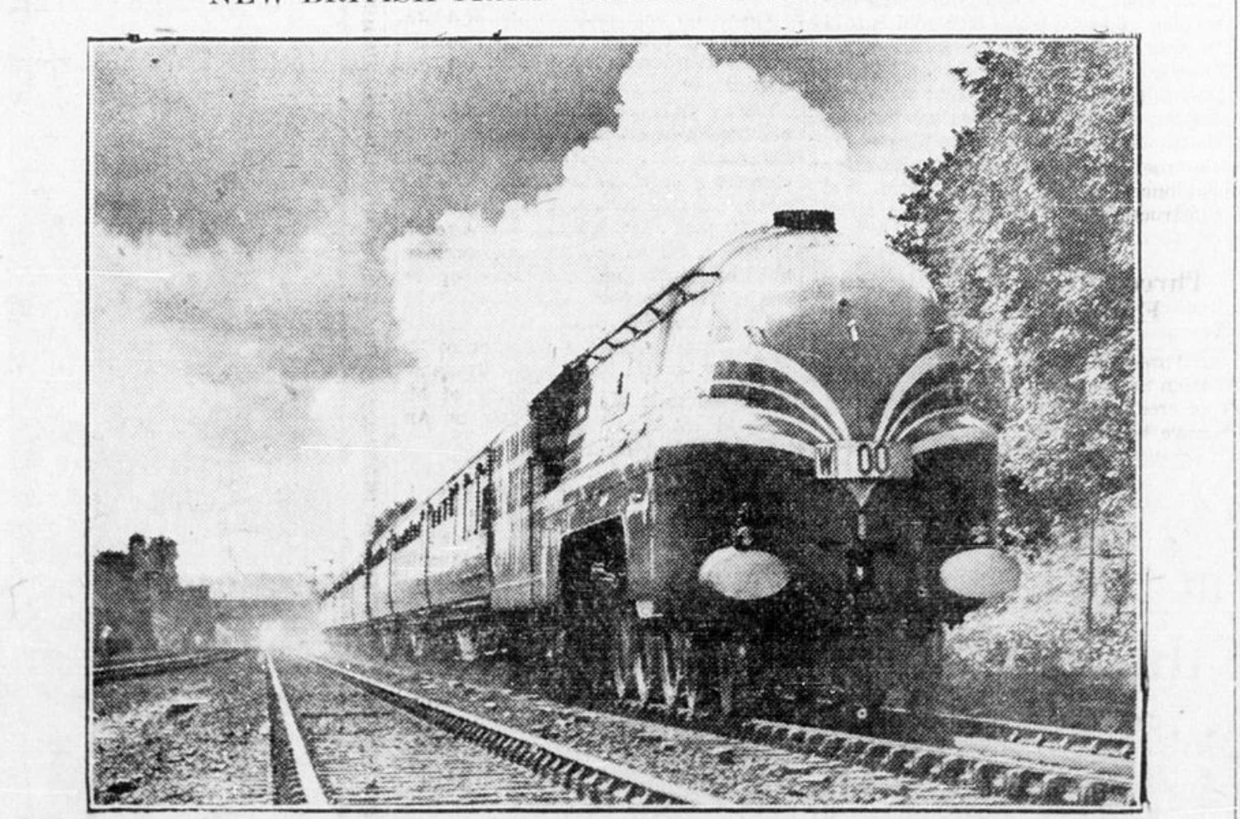
Britain's new Coronation Scot streamlined train did not wait very long before starting to break records. In its first trial run it set up four new British records and one new world's record while on a 316-mile trip from London to Crewe and back. It achieved the highest speed ever known on railways of the British Empire when it touched 114.4 m.p.h. near Stafford. Covering the 159-mile return trip in one hour and 59 minutes—an average of 80 m.p.h.—the Coronation Scot set up a new world record for the longest stretch of sustained speed.
