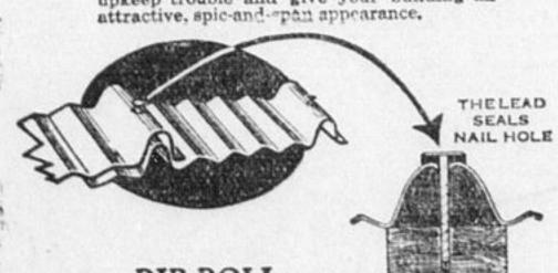
RIB-ROLL A "close-up" of Rib-Roll and the Preston Led-Hed Nail. Note the tight fitting, overlapeven a short distance away. Illustration shows the neat pattern which has been widely but
