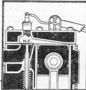
Note domed shape of combustion (H.C.) chamber above valves in Hupmobile engine. More power, greater smoothness are achieved through this development of the high-compression principle. Removable cylinder head also permits machining of inside of combustion chambers for exactly uniform size and shape.
