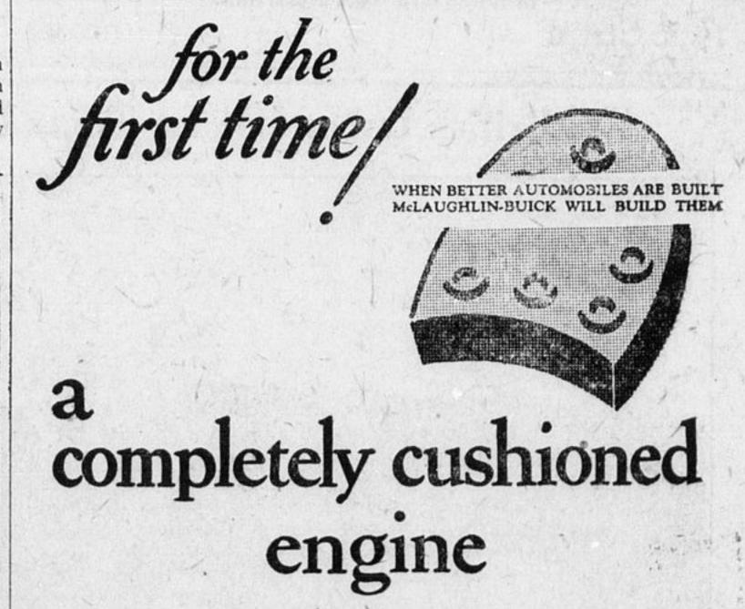
The McLaughlin-Buick Valve-in-Head engine now has "rubber heels." Here is an engine completely insulated and isolated from all metallic contact with its chassis. Thick rubber cushions, fore and aft, absorb
